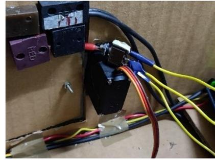
Figure 3 Servo motor for simulating door lock
