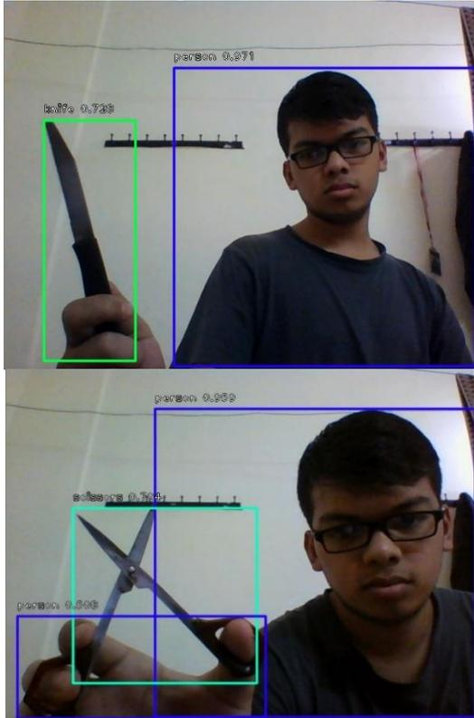
Figure 10 Weapons detected and labelled with their names
