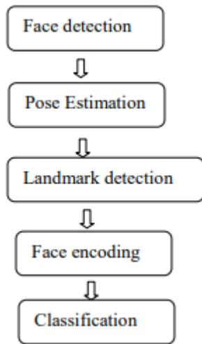
**Figure 5 Flowchart depicting face recognition pipeline**
