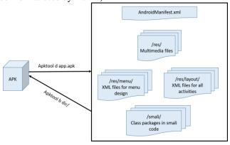
Figure 2: Diagram representation of Apktool decompile and compile option on any APK file
