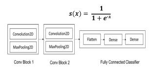
Figure 6: Structured of our used CNN network
