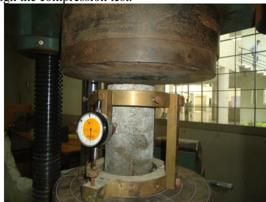
Fig:2 Setup of Compression Test
