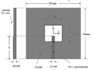
Fig. 4. Geometry of the microstrip printed wide-slot antenna with simple tuning stub
