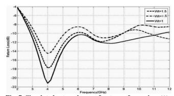
Fig. 7. Simulated return losses of antenna for various Wt.
