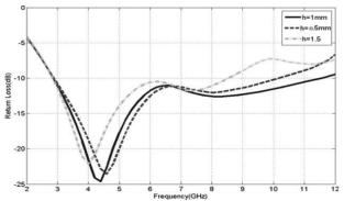
Fig. 5. Simulated return losses of antenna for various
