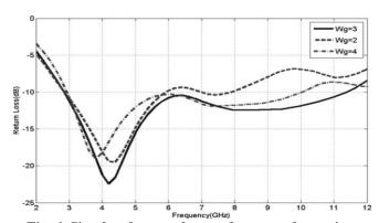
Fig. 6. Simulated return losses of antenna for various Wg.
