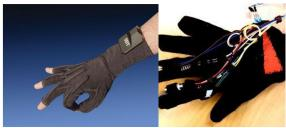
Figure 3 Glove Based Hand Gesture Recognition [9]
