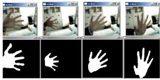
Figure 1 Hand Gesture Recognition in Rotation State [13]
