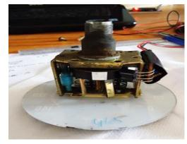
Figure 5. Optical sensor attached to odometer
