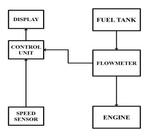
Figure 1. Block diagram
