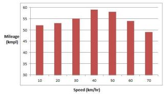
Figure 7. Mileage obtained during load condition of a singe person
