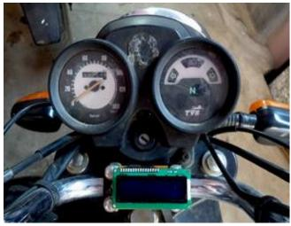
LCD mounted near the existing dashboard
