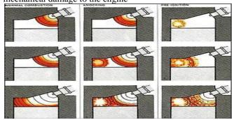
Fig: NORMAL COMBUSTION, KNOCKING, PRE-IGNITION
