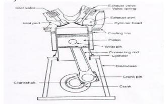
Fig. Air-cooled I.C. engine
