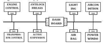
Figure 1. Automobile Subsystem With CAN
