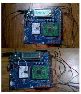
Figure 6. Two node CAN Communication
