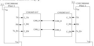
Figure 3. Hardware Connections for Implementing CAN
