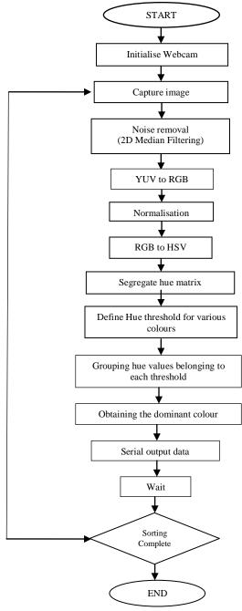
Fig. 2. OpenCV algorithm to obtain dominant colour The hue values are usually represented in degrees which range from 0 to 360. In HSV model, each of the primary colours is separated by  $120^{\rm O}$  and each of the secondary colours are separated by  $60^{\rm O}$  from the primary colour.
