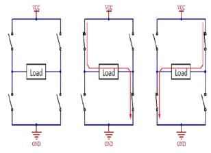
Fig. 4. H- Bridge showing connections for no output, +5 V and -5 V
