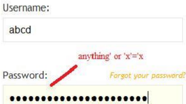
Figure [2]: Basic SQL Injection Attack
