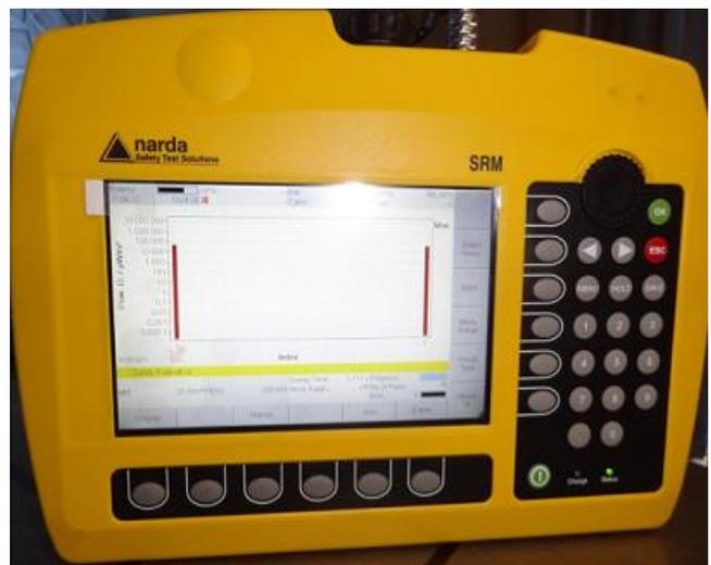
**Fig.-4 SRM-3006 Shows the readings in form of bar**
