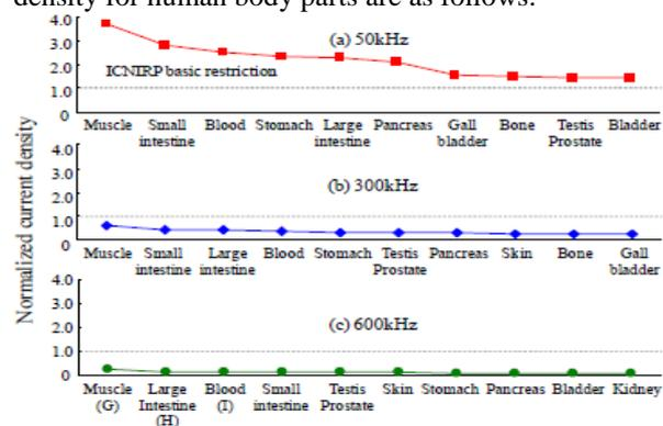
**Fig.1 The analysis results of normalized current density(maximum current density) ICNIRP basic restriction**
