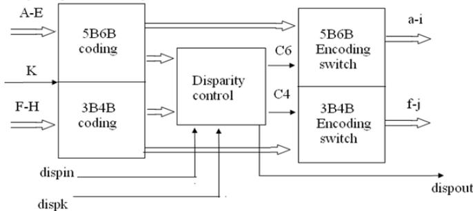
Figure.1: Block Diagram of Conventional 8B/10B Encoder
