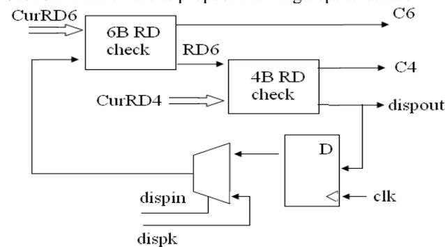
Figure.2: Block Diagram of Disparity Control
