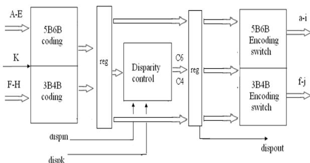
Figure.3: Block Diagram of pipelined 8B/10B Encoder Architecture
