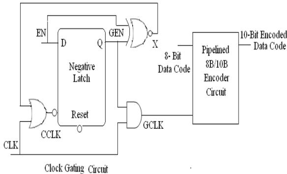
Figure.5: Pipelined 8B/10B Encoder Clock Gated
