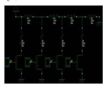
Fig 3.1: The Schematic layout of 4 bit R-2R ladder DAC
