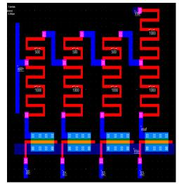
Fig 3.2: The Physical layout of R-2R ladder DAC
