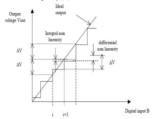
Fig2.3 : The illustration of integral and differential non-linearity
