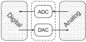
Figure 1.1: Data converters as interface between the analog and digital domain.
