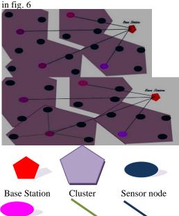
Fig. 6Concept of Initial Clustering Scheme
