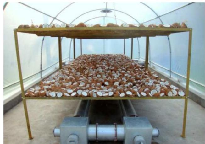
Fig. 7 Drying of Coconuts in Solar Tunnel Greenhouse Dryer Coupled with Biomass Backup Heater
