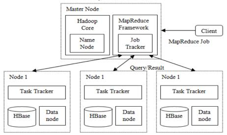
Figure 1: Architecture diagram for R.I. generation software using hadoop and hbase
