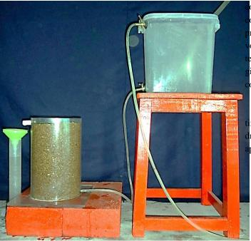
Fig 2 Hydraulic Conductivity typical test setup
