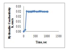
Fig 3.b Relationship between Hydraulic Conductivity and Time for Fine Sand -Dense state
