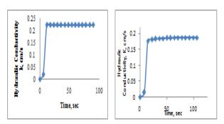
Fig 4. Relationship between Hydraulic Conductivity and Time for Coarse Sand - Loose Medium Dense and Dense
