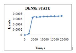
Fig 5. Relationship between Hydraulic Conductivity and Time for Quarry Dust - Loose Medium Dense and Dense state
