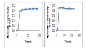
Fig 3.a Relationship between Hydraulic Conductivity and **Time for Fine Sand – Loose Medium Dense state**
