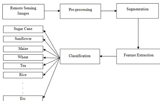
**Figure 1: General flow diagram for the crop identification system**
