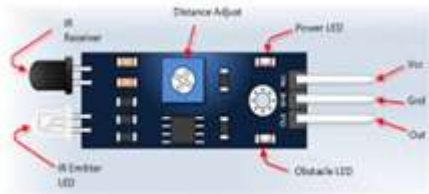
Fig.6.IR transmitter and receiver
