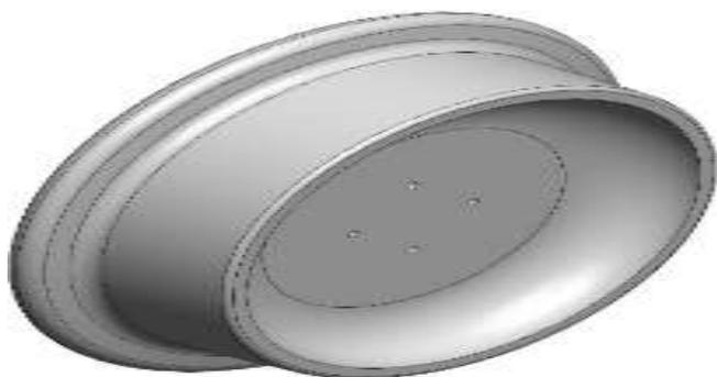
**Fig. 9. Design of rail wheel**
