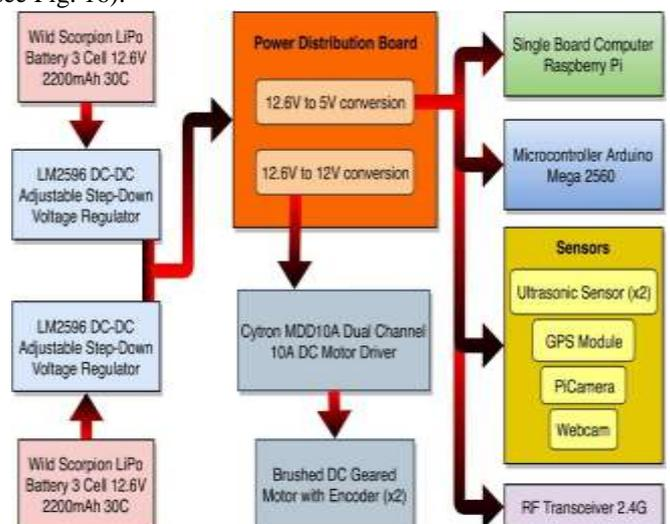
**Fig. 16. Block diagram of CARIV's electrical system**
