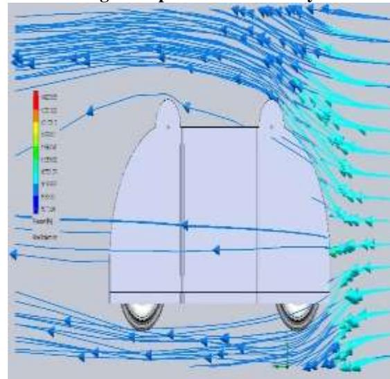
Fig. 7. Flow simulation of body
