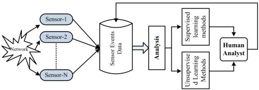
Figure-2: Working of IDS Architecture with Different Type of Sensors
