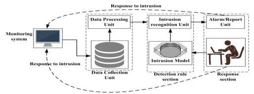
Figure-1 Intrusion Detection System Based Architecture
