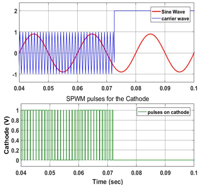
Fig. 4(a). SPWM pulses for the upper switches of the inverter
