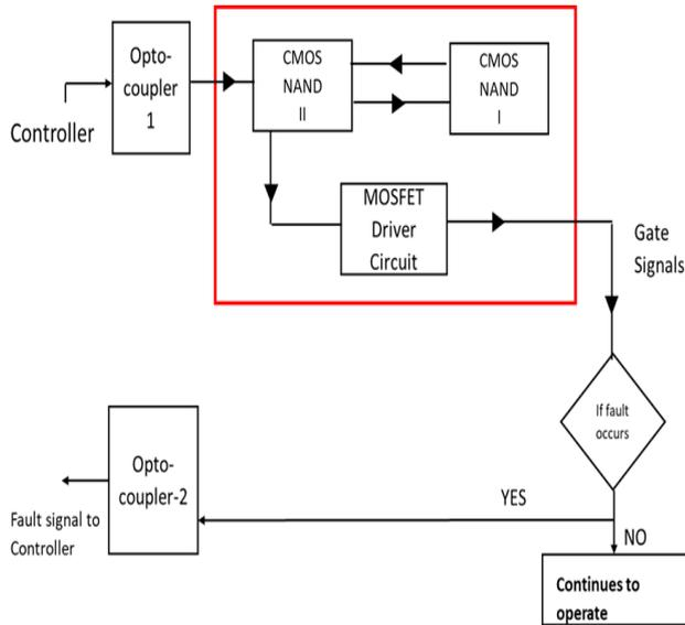
Fig. 1. Schematic diagram of the gate driver circuit
