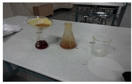
Fig. 4: Extraction phase. The combination of ginger and alcohol gets filtered by use of funnel and filter paper to get the pure solution with no solid inside.
