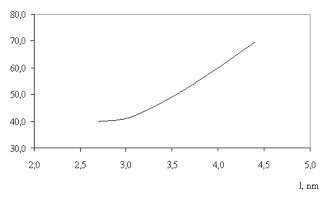
Fig. 4. Dependence Ids\_max(l) at Uds=Ug=0.5 V.
