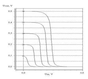
Fig. 5. The family of JSOMOSFET characteristics, where the Uds varies from 0.5 to 0.1
