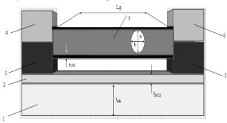
Fig. 2. Block diagram of an JSOMOSFET, where positions 1-6 correspond to figure 1, 7 joint oval working area. Here designations: Lg – gate length, a&b -large and small diameters of the joint working area, toxthickness of the sub-gate dielectric
