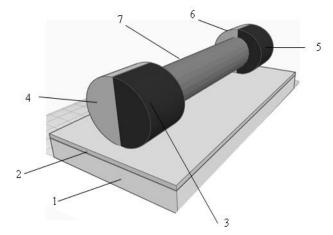
Fig. 1. Block diagram of an JSMOSFET, where 1- silicon substrate, 2- silicon oxide, 3 - n + - source, 4-p+ - source, 5-n+ - drain, 6-p+ - drain, 7-joint working area
