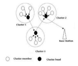
Fig..5. Heterogenous Network Clustering Model
