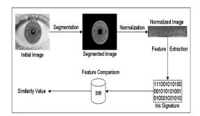
Fig. 1. Image Processing Method
