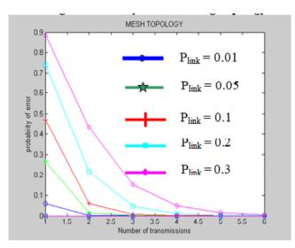
Fig.8. Probability Error for Mesh Topology
