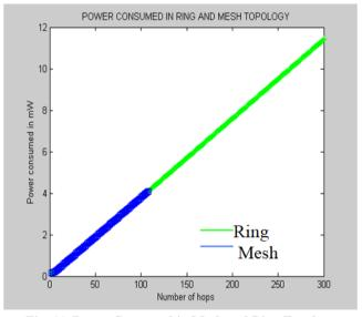
Fig. 11. Power Consumed in Mesh and Ring Topology
