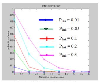
Fig.6. Probability Error for Ring Topology
