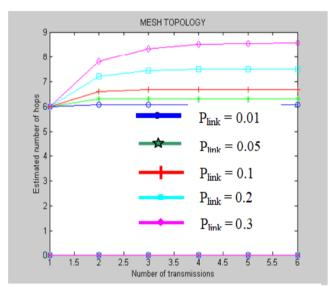
Fig. 9. Estimated Numbers of Hops for Mesh Topology
