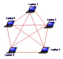
Therefore mesh topology provides reliable communication. In mesh topology the size of the network can be increased based on the user applications that is mesh topology is scalable. The main disadvantage of this model is it consumes
