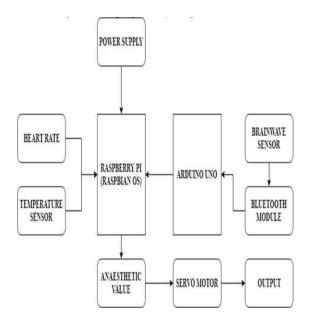
Fig. 1 Block Diagram for Automated Anesthesia Administration
