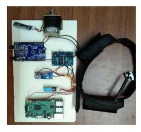
Fig. 3 Experimental Setup for Automated Anesthesia Administration
