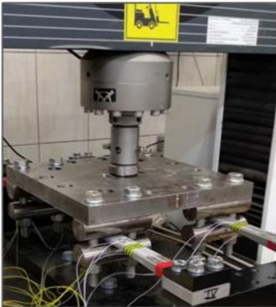
Figure 2. Tests on a bench for bending metal levers
