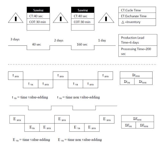
Figure 3 VSM according and schematic representation of value-adding and non value-adding input of time and energy
