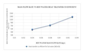
Fig. 3. Mass flow rate of hot water vs Hot water heat transfer coefficient
