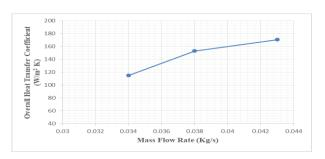
Fig. 4. Mass flow rate vs over all heat transfer coefficient
