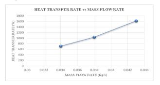
Fig. 5. Heat transfer rate vs Mass flow rate
