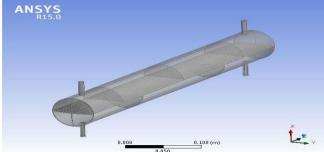
Fig. 1. 3 D Design of the heat exchanger
