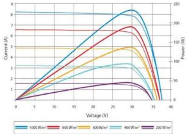
Fig-8. PV & IV Characteristic of MPPT Controller
