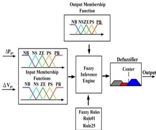
Fig:-5. Block diagram representation of Fuzzy Controller
