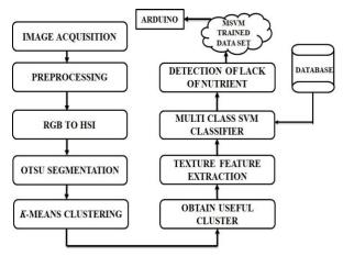
Fig. 5.Flow Chart of Image Processing Technique
