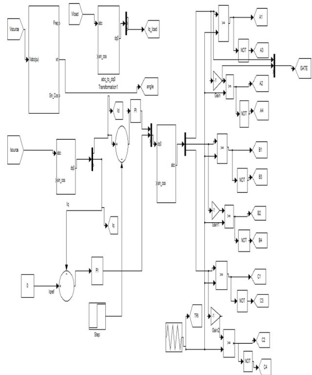
Figure 8. Simulink Model for PWM Switching Strategy of 7 Level CHB Inverter
