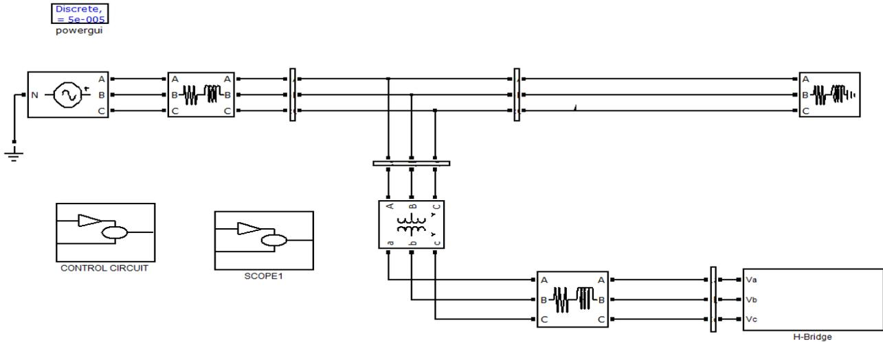
Figure 5. Simulink Model for 3 Phase Seven Level CHB Inverter
