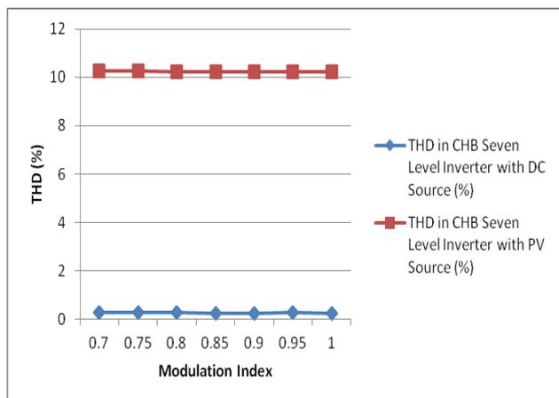
Figure 12. THD (%) in CHB Seven Level Inverter
