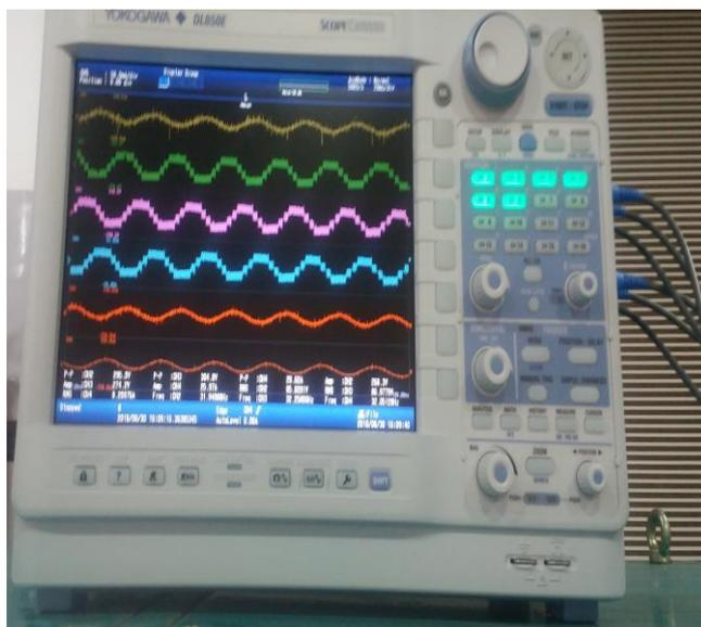
Figure 14. Voltage and Current Waveforms of Seven Level CHB Inverter on DSO
