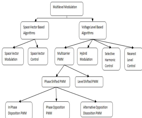
Figure 4. Multilevel Modulation Techniques
