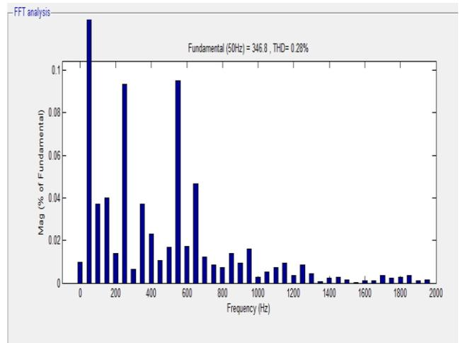
**Figure 10. FFT Analysis of designed 7 Level CHB Inverter with DC source**
