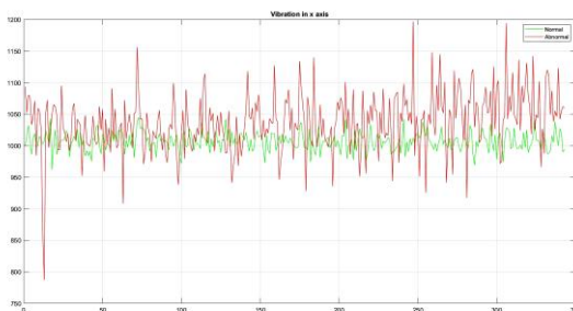
Fig 6: Vibration signatures for normal machining(green) and machining with lubrication error(red) in x axis
