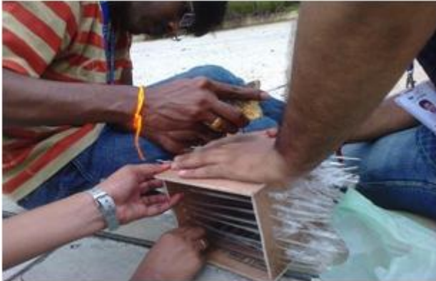
Fig.3. Insertion of optical fiber in concrete mould.
