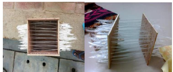
Fig.2 Wooden moulds with optical fibers.
