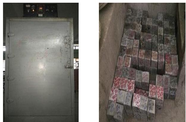
**Fig.3. Oven curing at 700C & Ambient curing**
