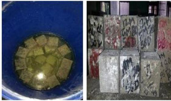
Fig.19. Cubes kept in sulphuric acid medium
