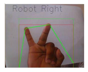
Fig. 6. Two dots to turn the robot right
