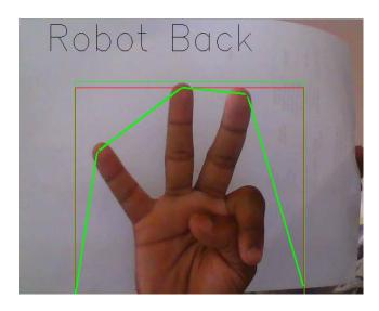
Fig. 8. Three dots to move robot backwards
