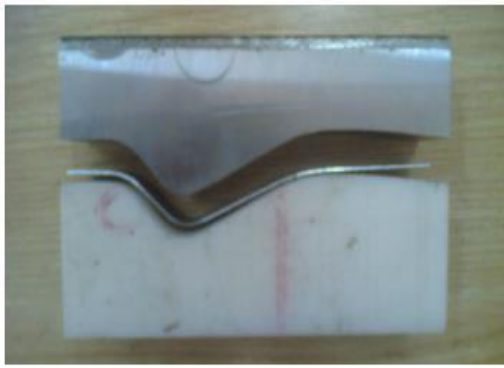
Fig 9: The asymmetric channel forming test
