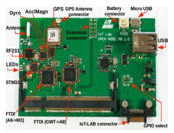
Fig.6 ARM Cortex combine with STM32 node point.
