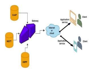
Fig. 4 Muti-protocol interfacing architecture
