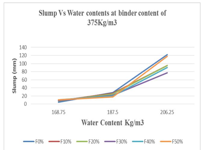
**Fig. 3. Slump and Water contents at binder content of 375Kg/m<sup>3</sup>**
