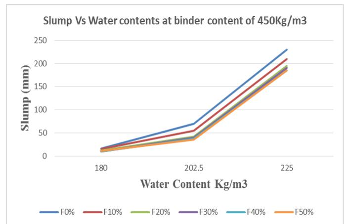
**Fig. 4. Slump and Water contents at binder content of 450Kg/m<sup>3</sup>**
