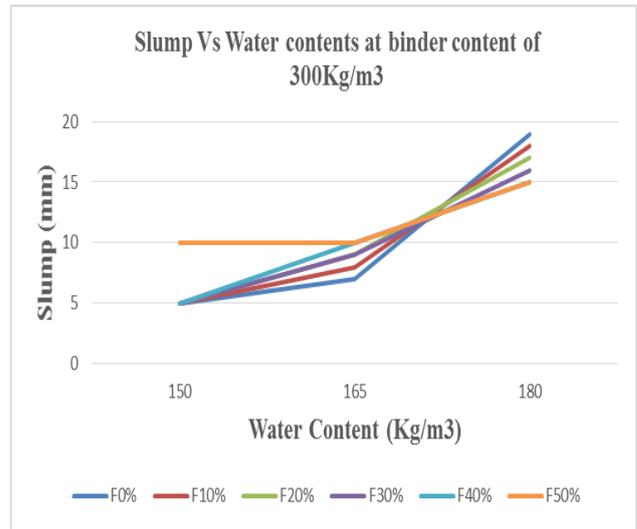
**Fig. 2. Slump and Water contents at binder content of 300Kg/m<sup>3</sup>**
