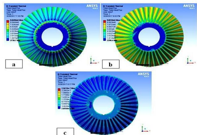
**Figure 3 Total heat flux in steam turbine impeller blades of 10.0 mm, 15.0 mm and 20.0 mm thickness.**
