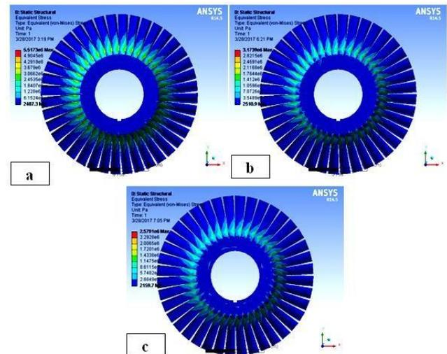
**Figure 2 Equivalent Von-Mises stress distribution in steam turbine impeller blades for the blade of 10.0 mm, 15.0 mm and 20.0 mm thickness.**
