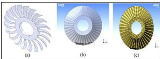
**Figure 1 Steam turbine impeller with blades (a) Comprehensive three-dimensional model (b) Inclusive ANSYS imported model (c) Complete ANSYS meshed model.**
