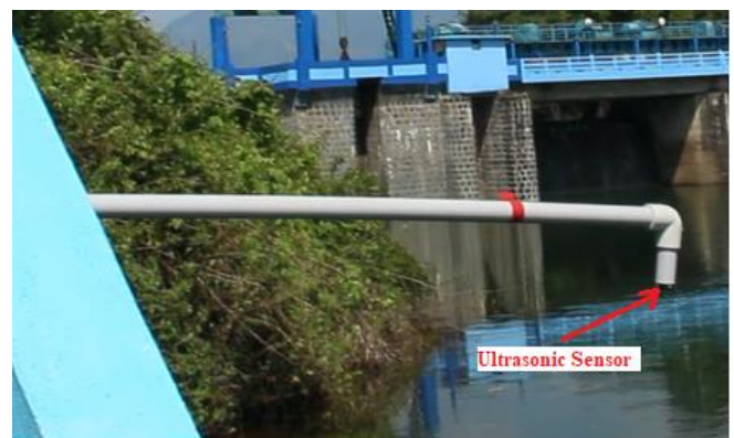
Fig.4. Ultrasonic Sensor Fixed on the Tip of the Pipe.
