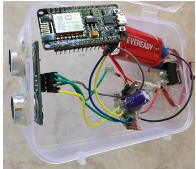
Fig.8. Hardware for Gate Position Measurement
