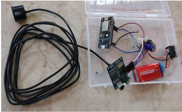
Fig.5. Hardware for Reservoir Level measurement
