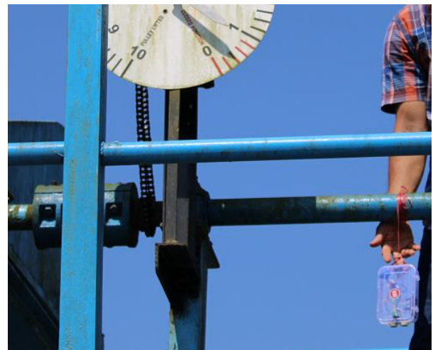
Fig.9. Ultrasonic Sensor Module Fixed on the Rotating Unit
