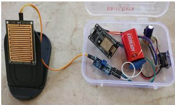
Fig.13. Hardware for Rain Measurement
