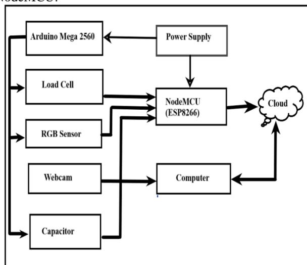
Figure1 Block Diagram for Non-Invasive Fruit Analyser\_1.7
