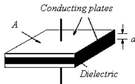
**Figure 3 Parallel Plate Capacitor**
