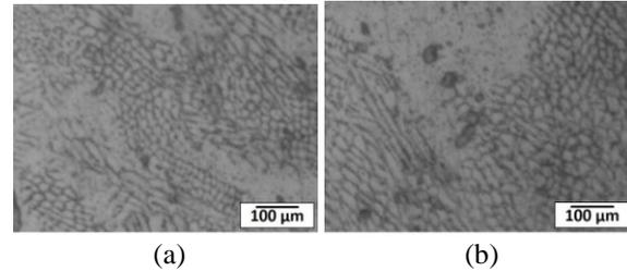
Fig. 3 OM image of (a) LW5 and (b) LW8 across the weldment
