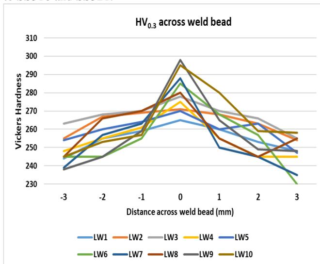
Fig. 5: Vickers Hardness across weld bead
