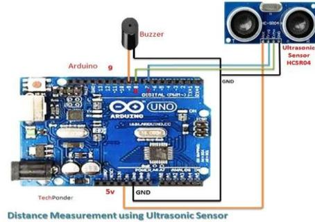
Ultrasonic Sensor Interface With Arduino
