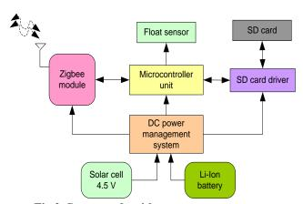
Fig.2. Sensor node with power management
