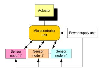
Fig.3. Cluster head mode C. Sink node
