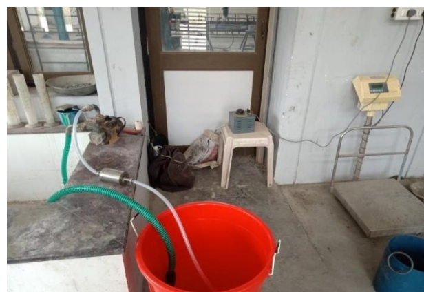
Figure 2. Experimental Setup of Magnetized Water System
