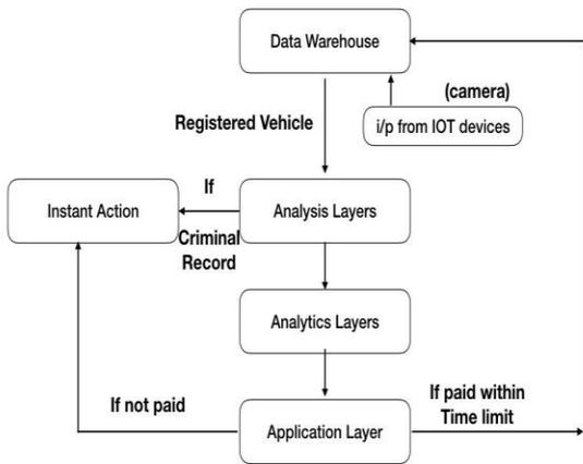
Fig. 2.2: Automatic Challan Generation Architecture
