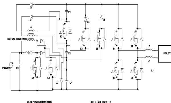
Fig: 2 Proposed Nine Level Solar Power Generation System
