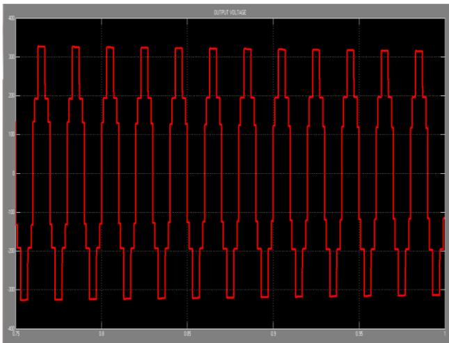
Fig 6.4 Output Wave Form of Four Level Waveform
