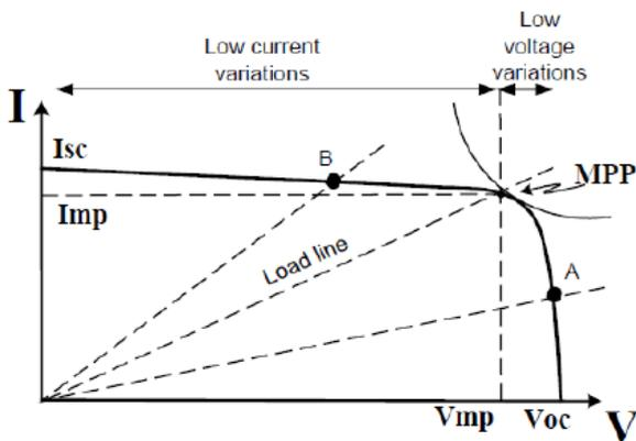
Fig 3 Graph with Voltage and Current
