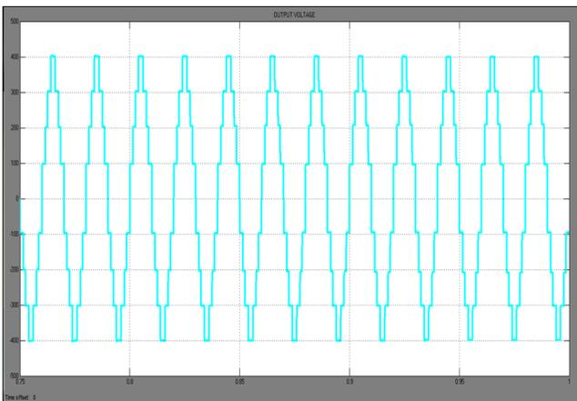
Fig 6.5. Proposed Nine Level Output Waveform
