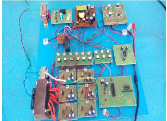
Fig 7.1 Hardware setup of nine level inverter system
